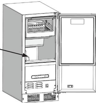
Pour cleaning solution slowly onto the front edge of evaporator plate behind the grid cutter.
