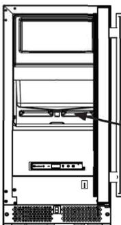
Remove the black reservoir drain plug from the bottom of the reservoir.
