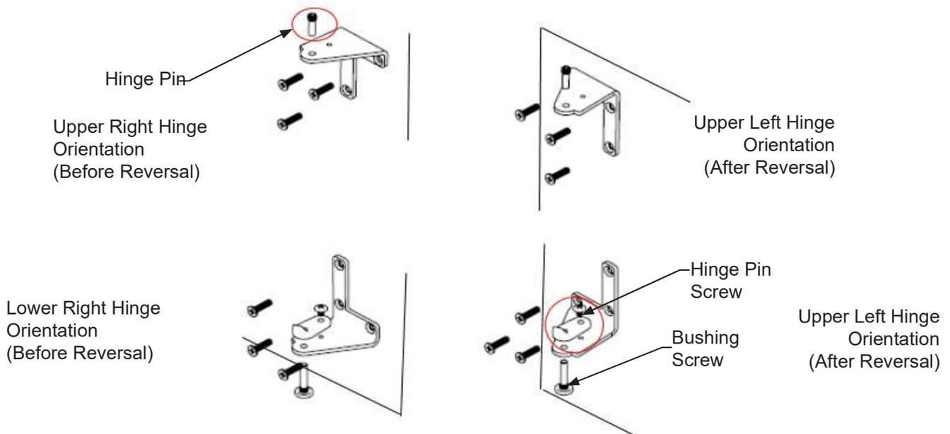
5. Using a 5/32" Hex Key, remove the Upper and Lower Hinge Brackets from the door, saving all components. Remove black plugs from opposite side of door. flip the Upper Hinge Bracket and reattach the Hinge Bushing and screw into place on the opposite side of the door (where plugs were removed). Remove the Cam Closer from the Lower-Hinge Bracket and attach it to the opposite side.
