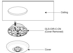
Place the cover on the device and twist to secure. Align the arrows on the device with the arrows under the cover. Twist the cover clockwise. The cover snaps into place.
