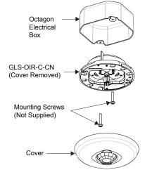
Place the cover on the device and twist to secure. Align the arrows on the device with the arrows under the cover. Twist the cover clockwise. The cover snaps into place.
