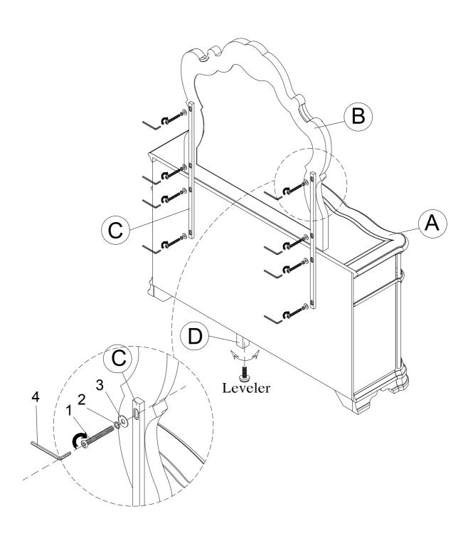
Place the Mirror (B) on the top of Dresser(A). Attach the Mirror (B) to the Dresser (A) with connecting stretcher (C), using Bolt (1), Spring Washer (2), Flat Washer (3), secure by Allen Key (4). Assembly product is now completed.
