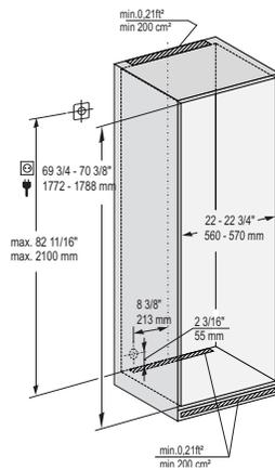
This is a fully integrated refrigerator-freezer appliance designed to be completely enclosed in a dedicated kitchen cabinet. This dedicated cabinet box must be constructed in accordance with the specified dimensions and must allow for sufficient air circulation to ensure proper operation. For more details about ventilation requirements, please refer to the Design Guide.
