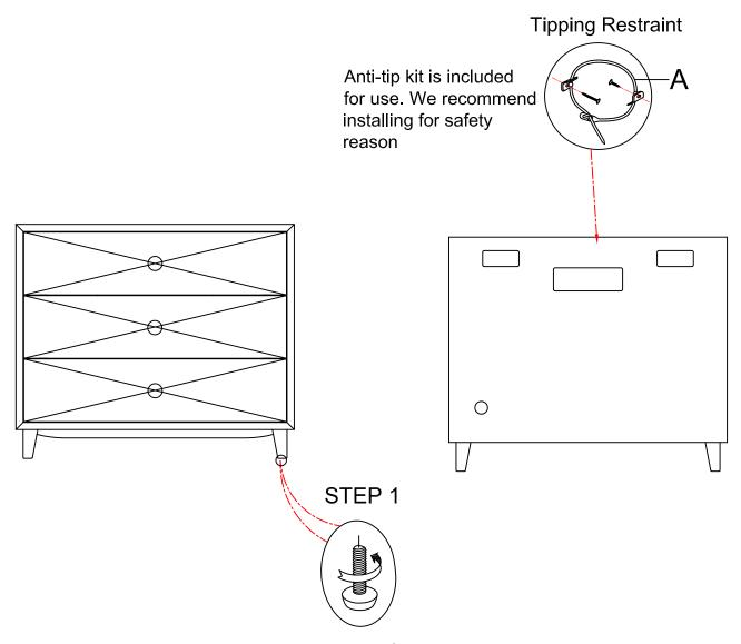
Adjust Leveler if needed to level case on uneven floor.
