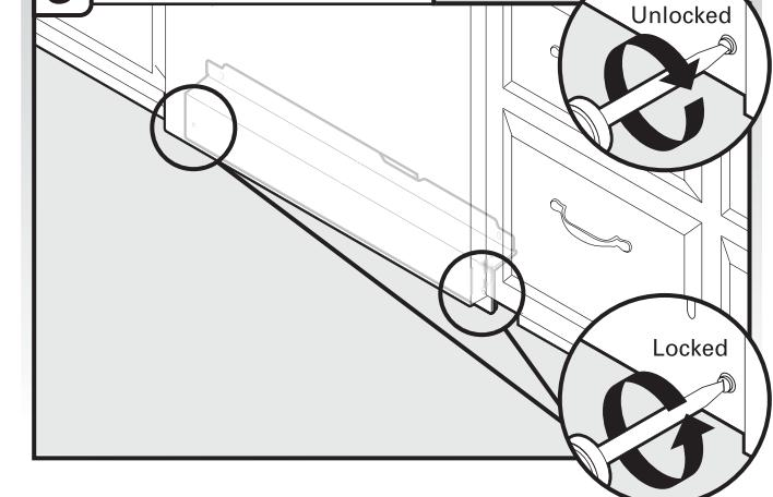
Using a flat-blade screwdriver, turn the fasteners  $\frac{1}{4}$  turn to lock into place. The fastener's slot will be straight up and down when properly locked.
