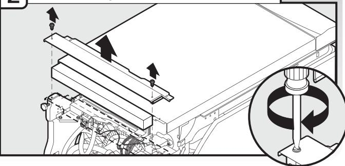
Using a flat-blade screwdriver, turn the plastic fasteners  $\frac{1}{4}$  turn to unlock them. Remove panel.
