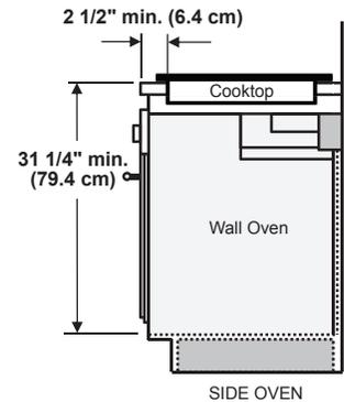
**IMPORTANT:** Maintain a minimum distance of 31 1/4" from the top surface of the countertop to the wall oven platform to ensure that the cooktop and wall oven do not interfere with each other (see picture).
