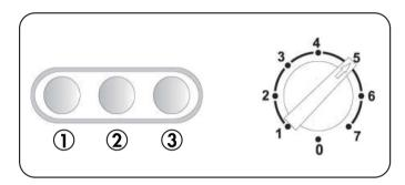
If the temperature control knob sets to 7, the compressor may run continuously. It's a quick
