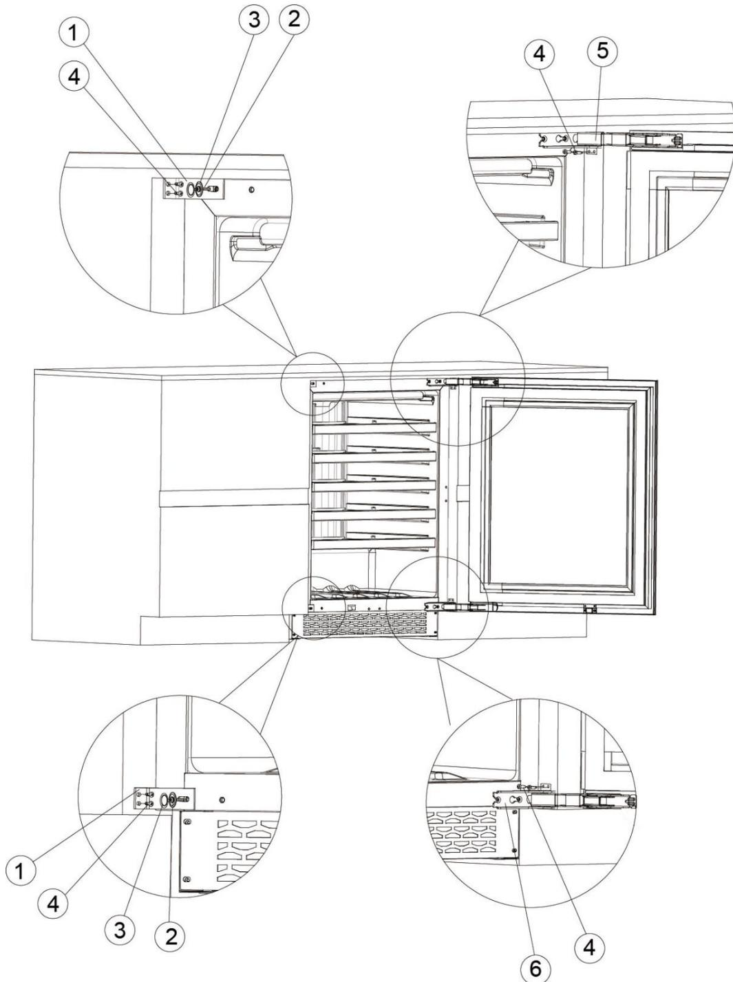
5. After adjusting the door panel, take out 4pcs ST4x35 self-tapping screws from the accessory bag, open the door seal, drill the screws through the screw holes on door frame, and tighten the door panel.
