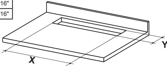
The minimum distance between the opening for the cooktop and the one for the hood must be of at least 1 3/16" - 1 15/16" according to the strength of the material used for the working top.
