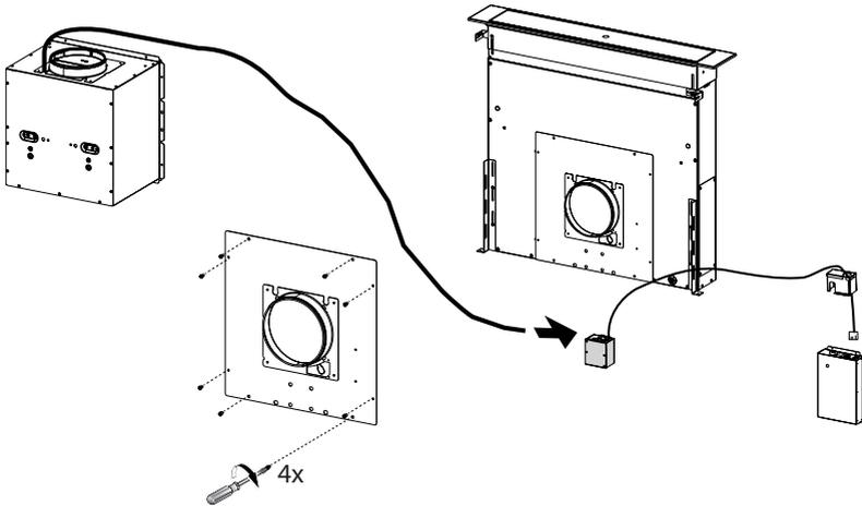
Connect the Remote Blower wiring to the connector of the Electric Unit.
