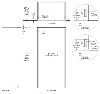
NOTE: 31/2\* (89) finished returns and shaded areas will be visible and should be finished to match cabinetry. Shaded line represents profile of unit with 3/4\* (19) panel.
