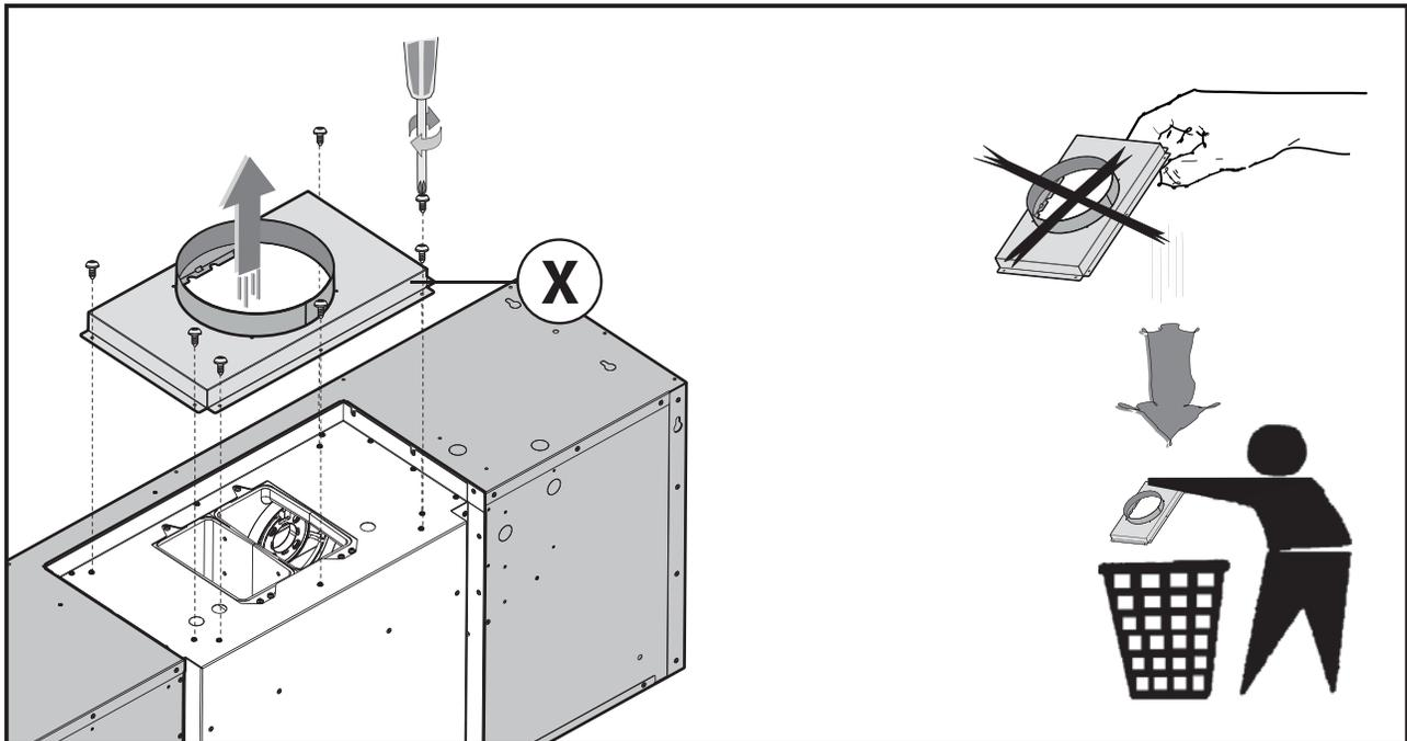
**Fig.1:** Take the circular shape **X** and fasten it to the hood using the 7 screws. To convert this model from the suction to the filtering version, it is not necessary to use the circular shape **X**.
