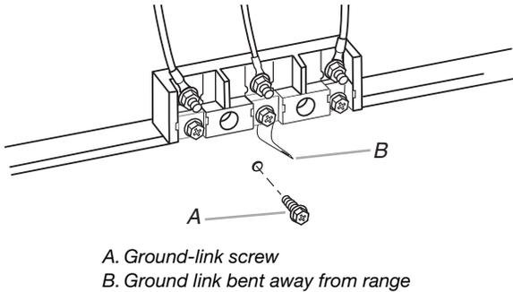
2. Connect the green ground wire from the power supply cord to the range using the ground-link screw. The ground wire must be attached first and must not contact any other terminal.
