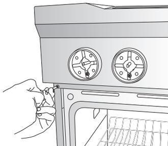
**NOTE:** Make sure to leave oven door open or the control console will not rest in the side brackets properly once it is detached.
