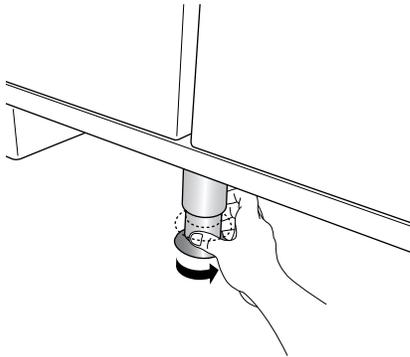
**NOTE:** This support is used only for shipping and is not needed for installation.
