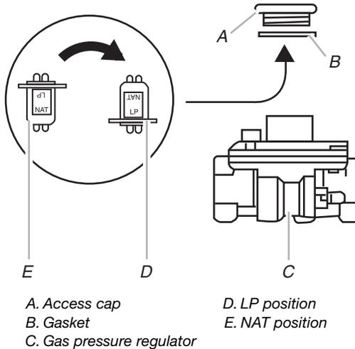
3. Test the gas pressure regulator and gas supply line. The regulator must be checked at a minimum 1" (2.5 cm) water column above the set pressure. The inlet pressure to the regulator should be as follows for operation and checking the regulator setting:
