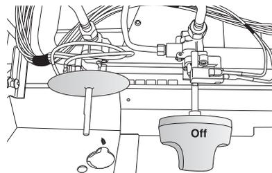
8. Turn the control knob to LO and using a butane extension lighter, light the burner.
