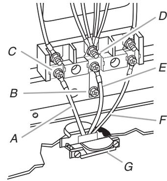
3. Connect the other 2 wires (lines 1 and 2) to the outer terminal screws on the terminal block.
