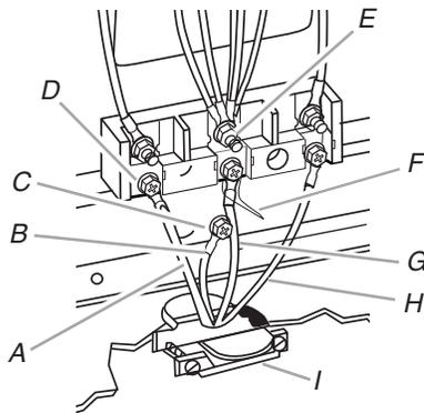
5. Connect the other 2 wires (lines 1 and 2) to the outer aluminum terminal blocks.
