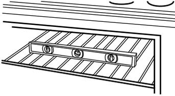
3. If range is not level, adjust the leveling rods. Turn leveling rods located behind the kick plate to level range and to raise or lower range to the desired countertop height.
