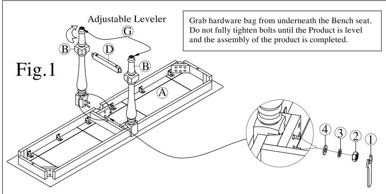
Step 1: Lay the Bench Seat (A) upside down on a flat soft surface. Insert Bench Center Leg (B) into Bench Seat (A), using the provided hardware as shown on Fig. 1. At the same time insert Side Stretcher (D) into bench Center Legs (B). Do Not Fully Tighten Bolts Yet
