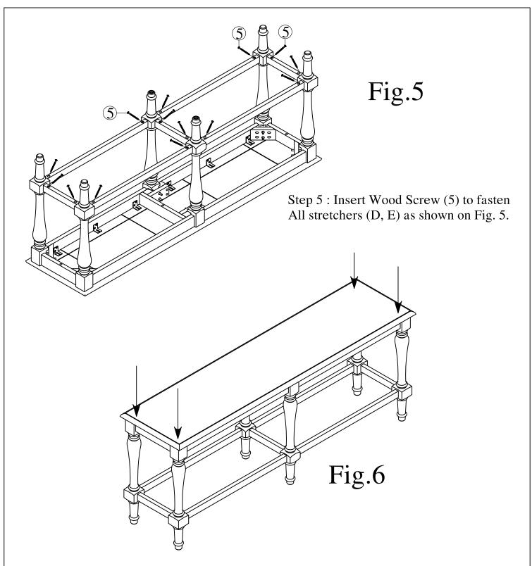
Step 6: Place the loosely assembled Bench on a hard flat surface and apply gentle downward pressure on the seat. As shown on Fig.6. Once the Bench is balanced and leveled, fully tighten all bolts.
