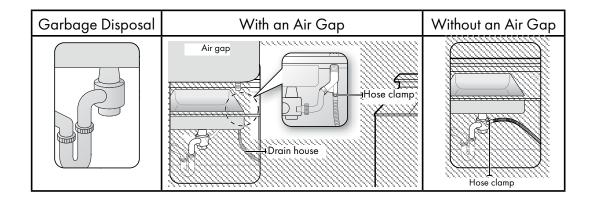
3. Check the size of the sink's drain hose connector. If needed, cut the drain hose so its end fits onto the sink connector (5/8", 3/4", or 1" as shown below). If the end of the drain hose does not fit onto the drain hose connector of the sink, use an adapter (not provided), available at any plumbing or hardware retailer.
