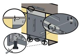
Using a level, be sure to check the dishwasher is level front to back and square to the floor and countertop.
