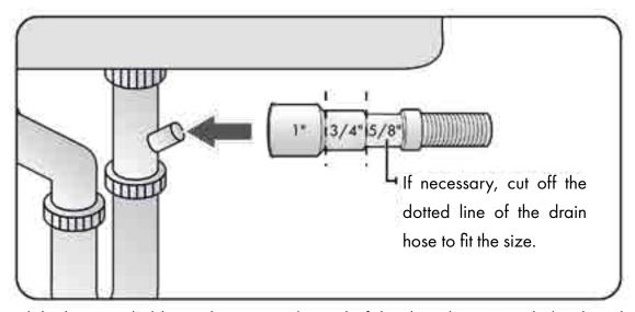
4. Slide the provided hose clamp over the end of the drain hose. Attach the drain hose to the sink connector, slide the hose clamp to the end of the hose, and then tighten the hose clamp.
