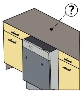
If the material (wood) under the countertop can be drilled or screwed into, align the brackets in this manner (below left).
