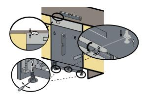
If the height of the enclosure is above 36" (914 mm), use the long leg supports as shown in the figure below.
