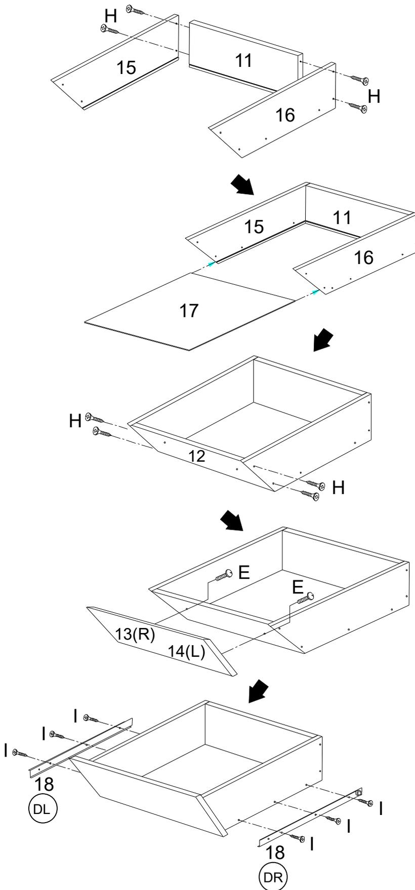
**Adjusting the bolts to align drawer outer front panel to fit drawer frame perfectly.**
