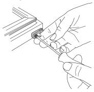
• To install the door, set the door onto the left bottom hinge pin. Holding the door in place, insert the new top left hinge pin into the door and secure the hinge to the case with screws.
