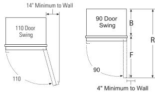
**NOTE:** Clearances are based on the recommended 2-1/4" handle standoff depth.
