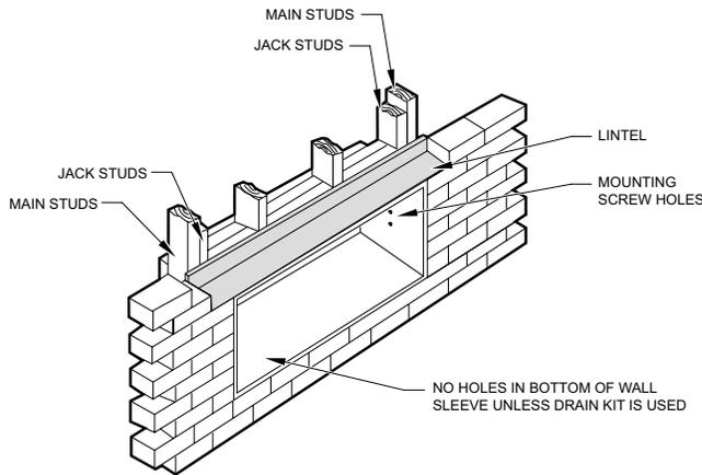
Note the use of a lintel under the first course of bricks above the wall sleeve. Do not use the wall sleeve as a lintel. The mounting screw holes shown are to be made by the installer.
