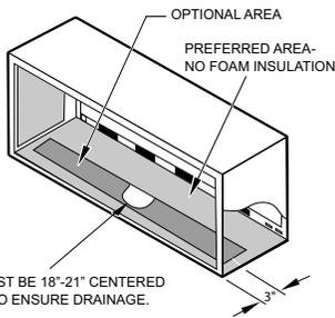
NOTE: IF THE DRAIN MUST BE LOCATED IN THE OPTIONAL AREA, THE FOAM INSULATION MUST BE CUT AWAY AND REMOVED TO ALLOW ACCESS TO THE DRAIN.
