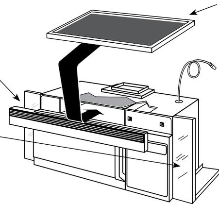
**Filter Kits JX81J-Recirculating Charcoal Filter Kit** To be used when the Spacemaker microwave oven cannot be vented to the outside.
