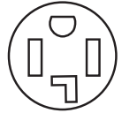
4-Wire Receptacle (14-30R)
