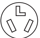
3-Wire Receptacle (10-30R)
