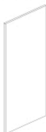
Anti-sweat foam ×1 Dimension: 18-1/8" x 1-5/16" x 9/16" (460mm x 846mm x 15mm)
