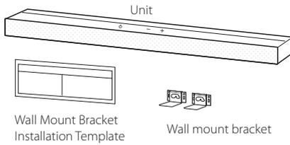
1. Match the TV's BOTTOM EDGE of Wall Mount Bracket Installation Template with the bottom of TV and attach to the position.
