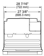
**CUTOUT DIMENSIONS - PROUD INSTALLATION IN WALL CABINET** 5 (127 mm) C 1" . (25 mm) Junction • FP FP Box Conduit 30" Opening (762 mm) 28 1/2" Min. (724 mm)< 29 1/8" Min. 23" 28 5/8" Max. (740 mm) (584 mm) (727 mm) 29 3/16" Max. (741 mm) 24" (610 mm) -6 31" (787 mm)
