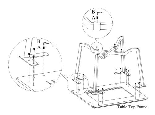
STEP 2: Put the table top frame face down on a soft surface, Attach the legs with X stretcher to the table top frame by using 20 bolts(A). Completely tighten all bolts. Turn the assembled table to the upright position.
