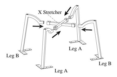
STEP 1: Insert the legs A and legs B to the X stretcher as shown.
