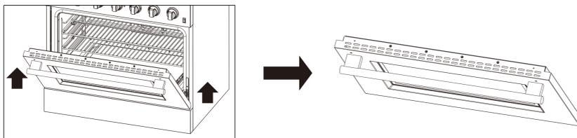
Step 3. Pull the original door outside of the oven.
