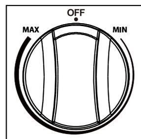
**IMPORTANT: To switch on, always lightly press the control knob inwards then turn.**
