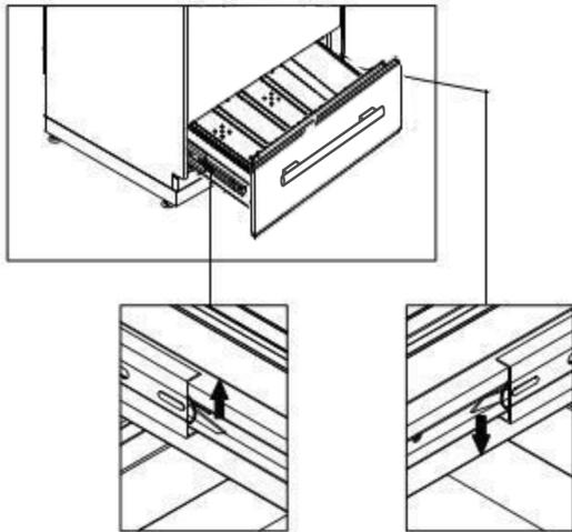
① Lift the left small hook upward, at the same time, push the right small hook downward.(see the picture )
