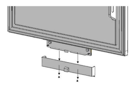
Remove FF Lower and Upper Bracket screws.
