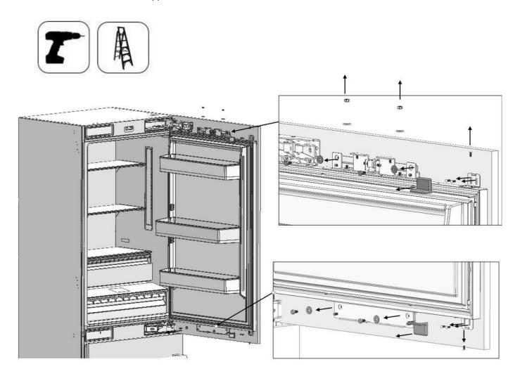
Remove the screw of FF Upper and Lower mechanisms.
