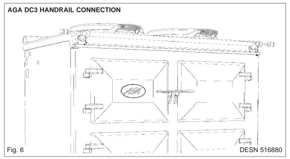
Slide the handrail through the handrail brackets.
