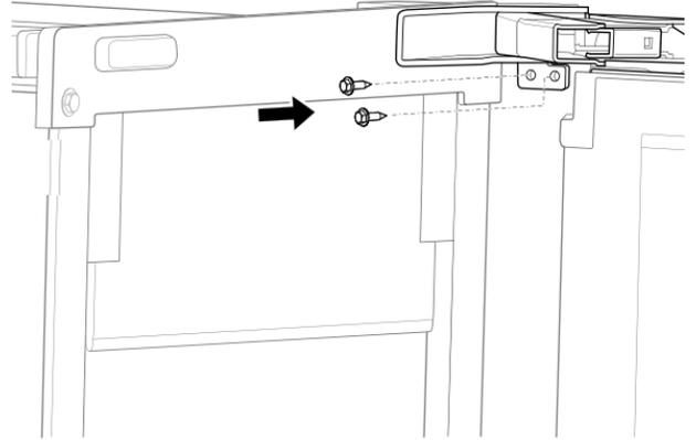
14. Attach the cabinet brackets (provided with ice maker) to the holes in the front of ice maker as shown in the illustration. Attach the cabinet brackets to the side of the cabinet with wood screws.
