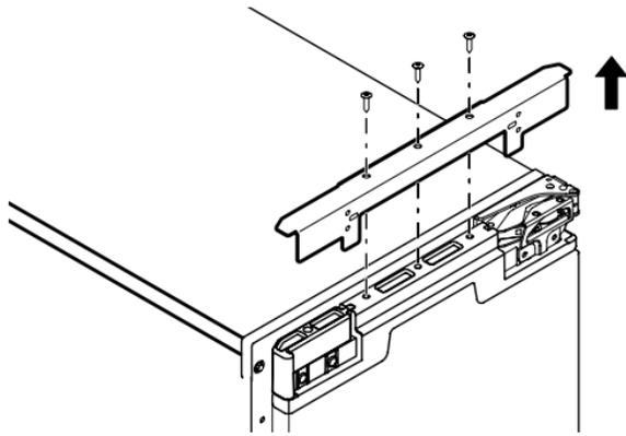
2. Remove the top and bottom end caps using the Phillips screwdriver and place them aside.
