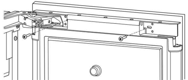
6. Adjust the panel side to side to achieve a desired gap on both sides. Install the remaining screws through the door bracket into the panel.
