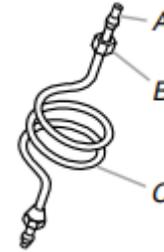
A. Compression sleeve C. Copper tubing
