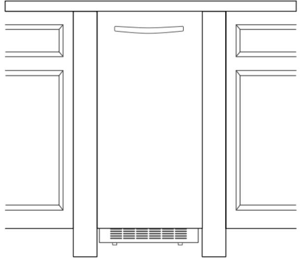
5. From inside the door, install the wood screws through the slotted holes in the metal brackets. Continue to step 11 in the "Leveling and Securing" section.
