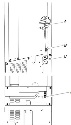
A. Copper tubing C. Inlet water tube clamp and supply line connector for standard model
