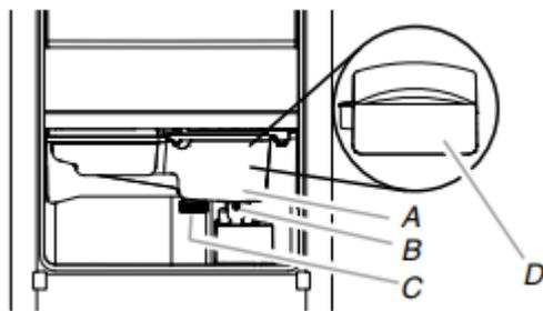
A. Water pan      C. Drain cap
