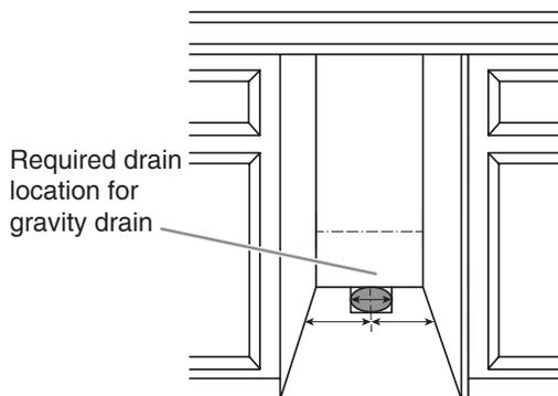
Required drain location for gravity drain
