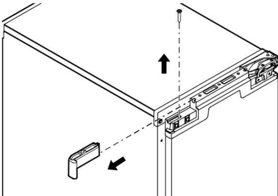
3. Reinstall top metal bracket using screws removed in step 1.
