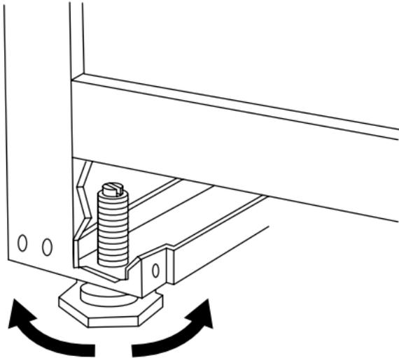
5. Push up on the top rear of the ice maker and locate the leveling legs that are on the bottom rear of the ice maker.
