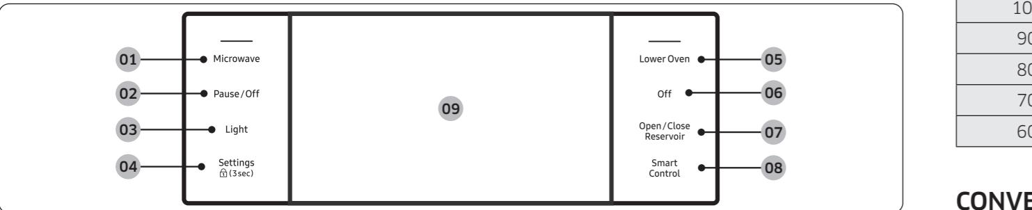
**01 Microwave**: Use to display the upper Microwave oven mode screen on the display. Touching here does not turn the oven on or off. It only displays its current status.
