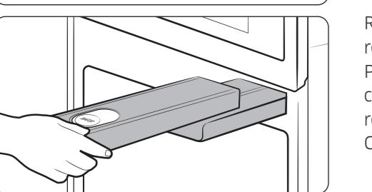
Replace the cap or the clear plastic top, and then slide the water reservoir back into the reservoir slot.
