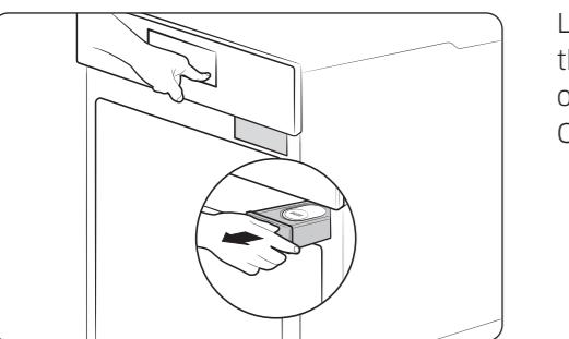
Locate the water reservoir. The water reservoir is on the right side of the oven, just above the oven opening. Touch **Open / Close Reservoir** on the control panel to eject the water reservoir.
