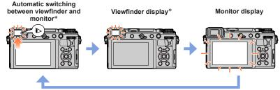
\* When [Eye Sensor AF] in the [Custom] ([Focus / Release Shutter]) menu is set to [ON], the camera adjusts the focus automatically as the eye sensor is activated. Even when [Eye Sensor AF] is set and the camera automatically adjusts the focus, a beep will not sound.
