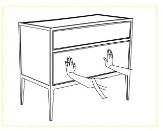
**WARNING!!!:**Do not push the drawer front with one hand only on end of the drawer front as shown in the photo.
