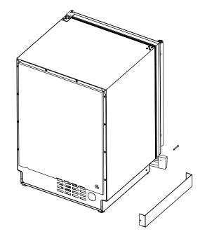
3. Align front hole wit hole in shell accessory, hole in base, and hole in grille. Tighten screw.
