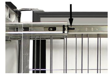
Press the left basket release lever down. At the same time, lift the matching right basket release lever up. Pull basket out until it is free of the tracks and the cabinet.
