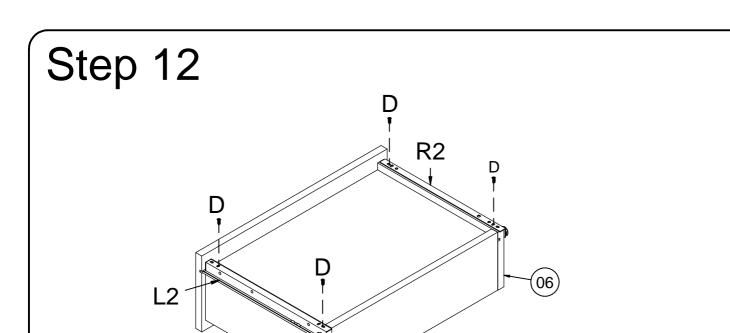
Attach slides (L2,R2) to parts (6,7) with screw (D).
