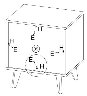
Secure back panel (9) using screw (E) and support (H).
