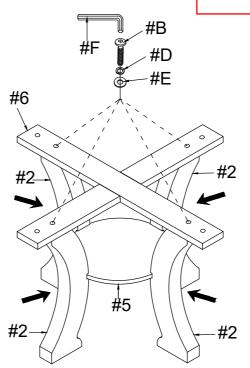
Align legs (#2) to the mounting plate (#6) and shelf (#5), then secure by using bolts (#B) with washers (#D,E).
