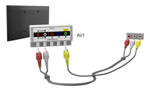
If you are using the TV's AV2 input connectors, use the included AV connection adapter to connect the device's audio and video output to the TV.
