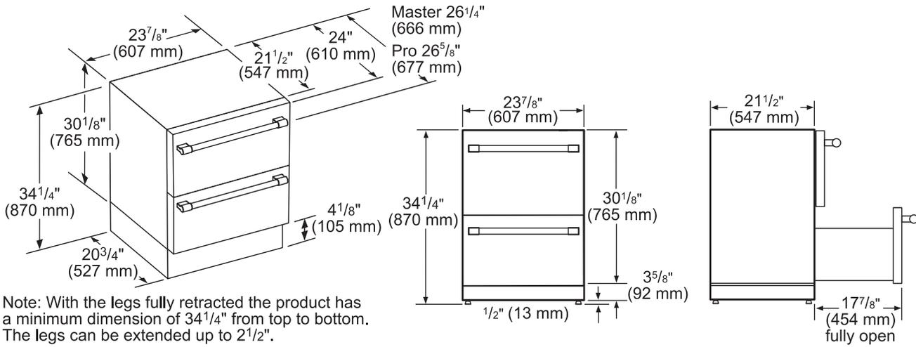
Note: With the legs fully retracted the product has a minimum dimension of 34<sup>1</sup>/<sub>4</sub>" from top to bottom. The legs can be extended up to 21<sup>1</sup>/<sub>2</sub>".
