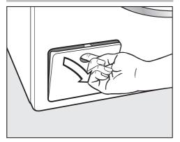
Open the access flap to the drain system.
