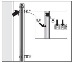
Secure the shipping struts to the back of the washing machine.
