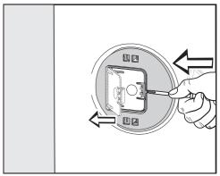
Press against the catch with a thin object (a narrow screwdriver, for example).
