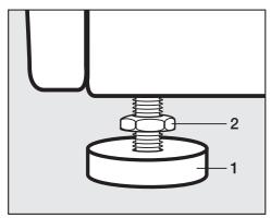
Using the wrench supplied, turn counter nut 2 in a clockwise direction. Then turn counter nut 2 together with foot 1 to unscrew.
