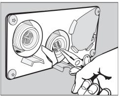
Use pointed pliers to grip the bar and pull out the filter; then clean the filter. Reassemble the appliance in reverse order.
