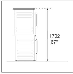
The washing machine can be installed as a washer-dryer stack together with a Miele Tumble Dryer. A stacking kit (APCL 001, optional accessory) is required for this.
