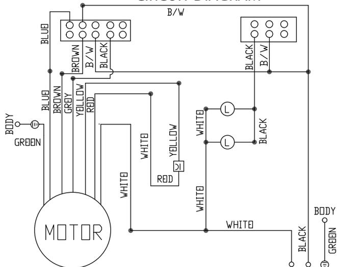
REMARKS: CONDENSER 4uF 250VAC FIT AC120V 60Hz
