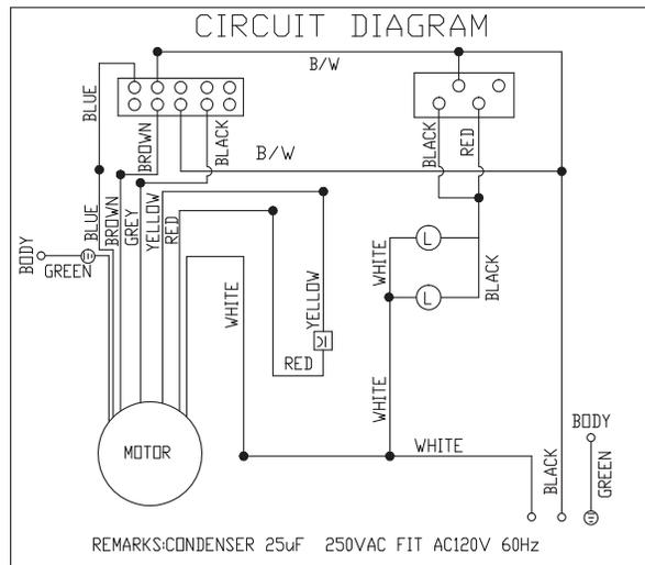
Diagrams – Fan Curve & Wiring
