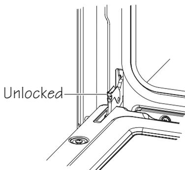
3 Grasp the edges of the oven door with both hands and push the oven door fully closed. Lift up and pull oven door toward you to remove. Set the oven door(s) aside on a covered work surface.
