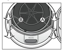
Use a T30 Torx screwdriver to unscrew the two screws on the base plate of the door hinge (A).
