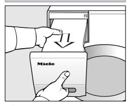
Remove the condensed water container.
