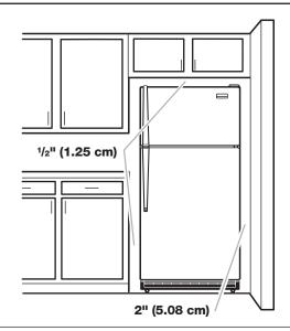
To ensure proper ventilation for your refrigerator, allow for a  $\chi'''$  (1.25 cm) space on each side and at the top. Allow at least 1" (2.54 cm) between back of cabinet and the wall. If your refrigerator has an ice maker, make sure you leave some extra space at the back for the water line connections.
