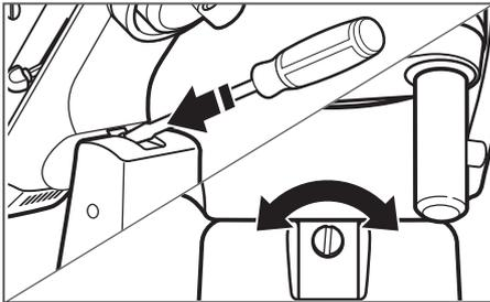
**(OPTIONAL) To adjust beater to bowl clearance:** Tilt the motor head back; then, using a flat-head screwdriver, turn the screw slightly counterclockwise (left) to raise the beater, or clockwise (right) to lower the beater. Adjust the beater so that it just clears the surface of the bowl. If you overadjust the screw, the bowl lock lever may not lock into place.
