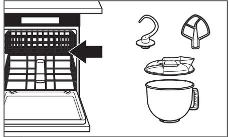
**2** Bowl, pouring shield\*, flat beater, and white dough hook may be washed in a dishwasher. Or, clean them thoroughly in hot sudsy water and rinse completely before drying. Do not store beaters on shaft.
