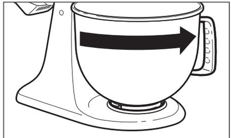
**3** **Remove the bowl:** Gently turn the bowl counterclockwise to release it from the bowl clamping plate.
