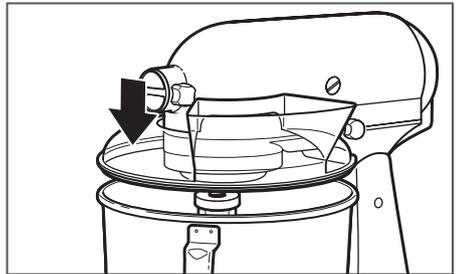
**(OPTIONAL) Place the pouring shield\*:** Slide the pouring shield from the front of the Stand Mixer over the bowl until the pouring shield is centered. The bottom rim of the pouring shield fits inside of the bowl. The pouring chute will be just to the right of the attachment hub as you face the Stand Mixer.
