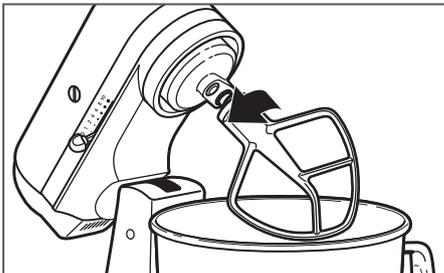
**2** **Remove the accessory:** Press the accessory upward as far as possible, then turn the accessory clockwise and pull it away from the beater shaft.
