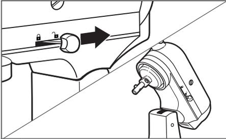
**1** **Raise the motor head:** Check to be sure that the Stand Mixer is unplugged, and the speed control is turned to "0"; then, slide the locking lever to the unlock position and lift the motor head.
