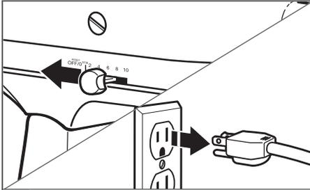
**1** Turn Stand Mixer off and unplug before cleaning. Wipe the Stand Mixer body with a soft, damp cloth. Do not use household/commercial cleaners. Wipe off the beater shaft frequently to remove any accumulation of residue. Do not immerse in water.
