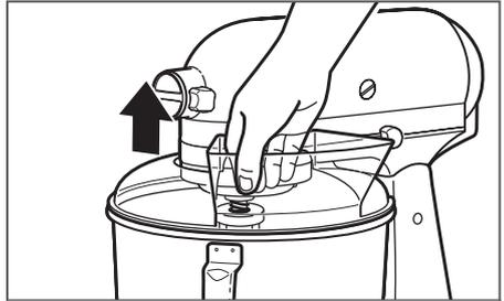
**(OPTIONAL)** **Remove the pouring shield\*:** Lift the front of the pouring shield clear of the rim of the bowl, and pull away from the Stand Mixer.
