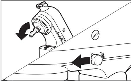
**5** Lower the motor head until it is all the way down, then slide the locking lever to the lock position. Before mixing, test lock by attempting to raise motor head.
