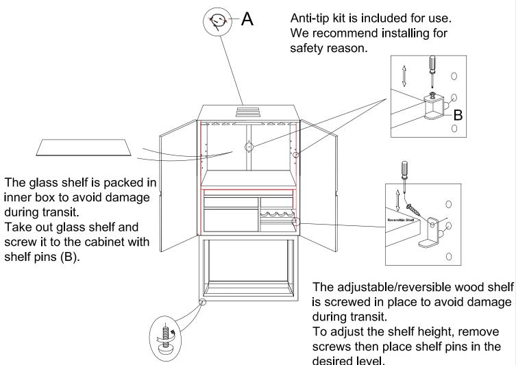
Adjust leveler if needed to level cabinet on uneven floor.
