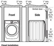
If washer and dryer are installed in same closet, door(s) MUST be vented with 120 sq.in. minimum louvered opening, equally divided, located 3" from top and bottom of door. Louvered door(s) with equivalent air openings for full-length of door is acceptable. Air openings MUST remain unobstructed with door(s) installed.
