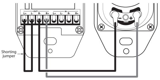
ISSP connected to one channel output with shorting jumper on the other channel
