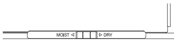
The Moist-Dry slide control allows you to open or close the vent slots in the door. The MOIST setting holds moisture in, while the DRY setting allows steam and moisture to escape from the drawer.
