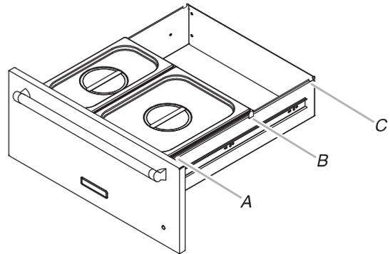
A. Position 1 pan support rail locator notch
