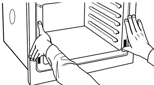
3. Push oven completely into cabinet and center oven into cabinet cutout.
