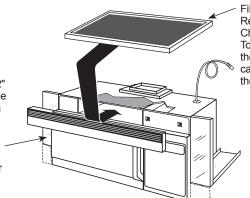
Filter Kit JX81H– Recirculating Charcoal Filter Kit To be used when the microwave oven cannot be vented to the outside.
