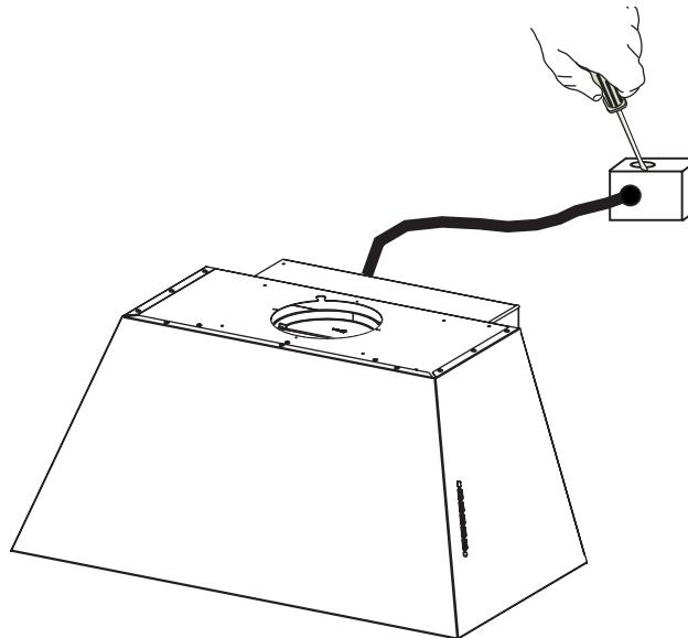
Remove the Wiring Box compartment cover by unscrewing the two screws.
