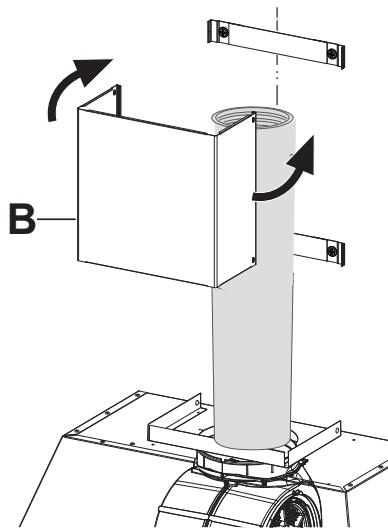
Slightly widen the two sides of the upper chimney and hook them behind the brackets, making sure that they are well seated.
