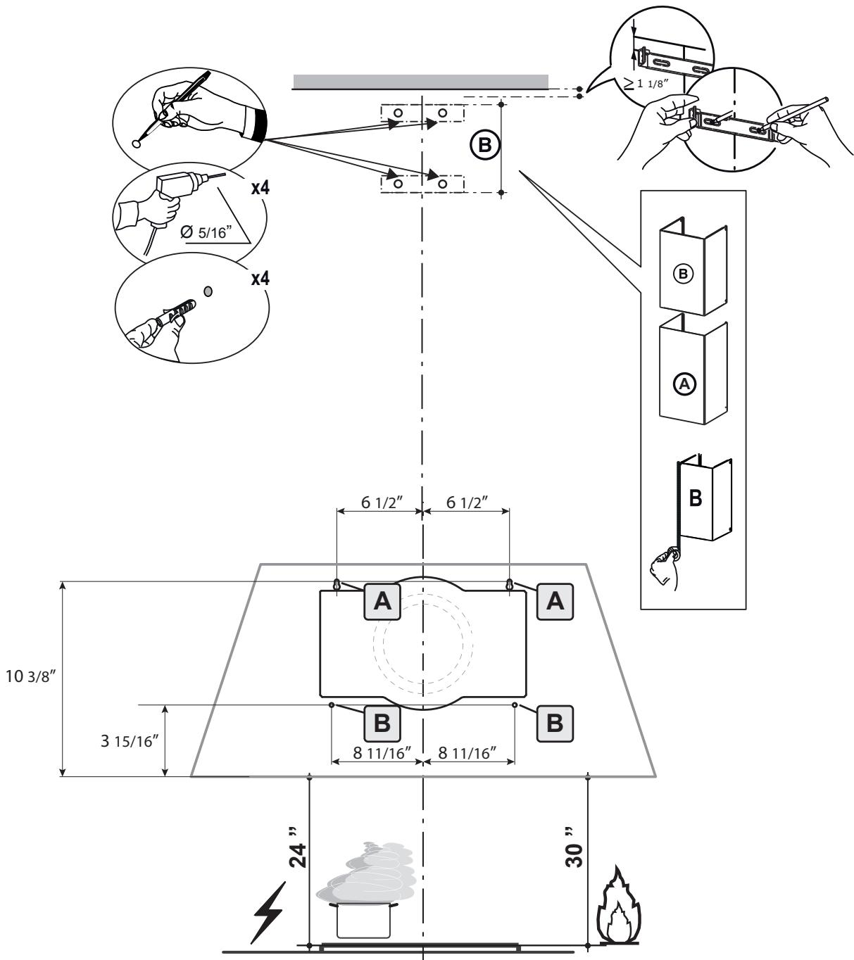
Mark the wall where indicated (A),  $10\frac{3}{8}''$  above the horizontal line and at  $6\frac{1}{2}''$  distance on the left and right of vertical line. Checking that the two marks are level.
