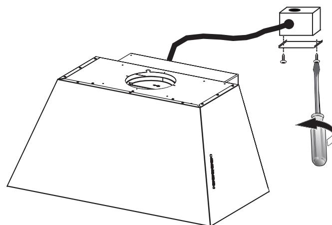
Pull the cable from the Power Supply through the Hole for the Electrical Connection to the Wiring Box.
