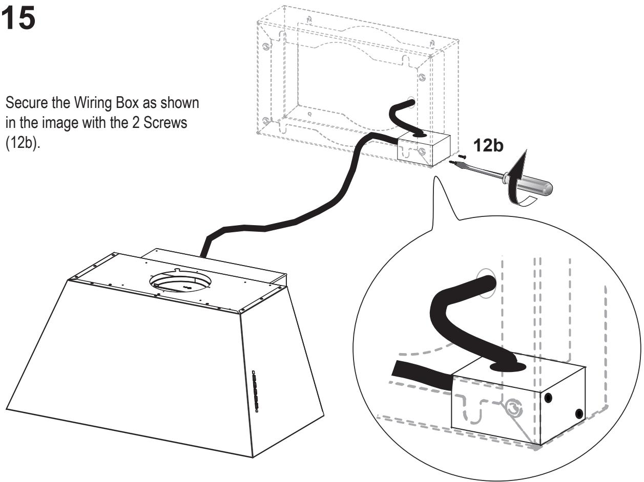
**Attention:** After the Wiring Box installation, place the Cable inside a Rear Section without stressing for the Cable.
