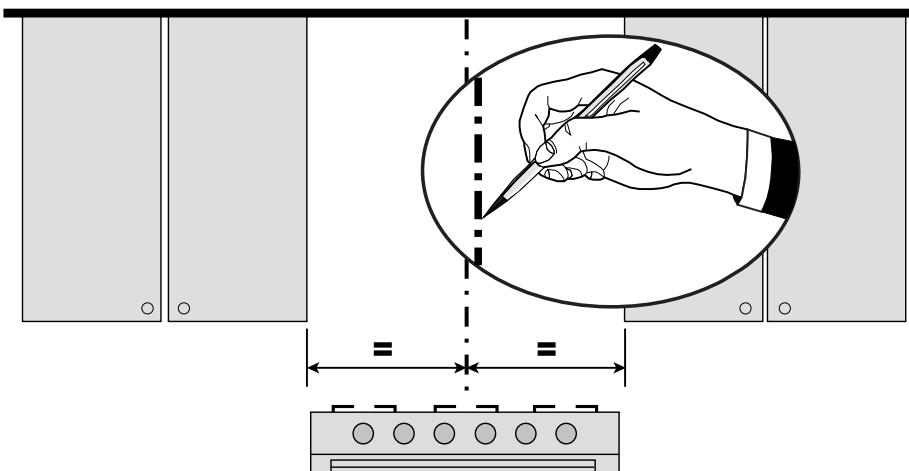
Draw a vertical line on the supporting wall as high as practical, at the center of the area in which the hood will be installed. Draw a horizontal line at where the bottom edge of the hood will be located as indicated in the figure that is a minimum of 24" above Electric cooking surface and 30" above Gas.
