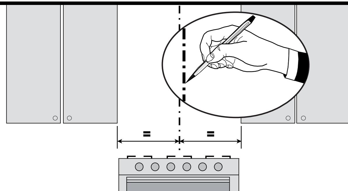
Draw a vertical line on the supporting wall as high as practical, at the center of the area in which the hood will be installed. Draw a horizontal line at where the bottom edge of the hood will be located as indicated in the figure that is a minimum of 24" above Electric cooking surface and 30" above Gas.
