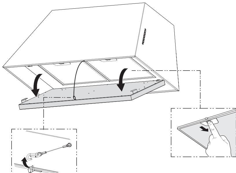
Open the panel, unlock the security cable as shown. Remove the filters by pushing the lever towards the back of the unit and at the same time pulling downward. Do not discard the filters and set aside for future use.
