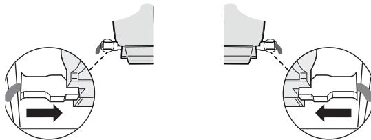
From inside the hood re-connect the Connectors on the left and right side shown in the image above.
