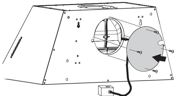
Fix the cover plate with the 4 screws removed previously and route the wiring box outside of the hood body through the notch on the cover plate.
