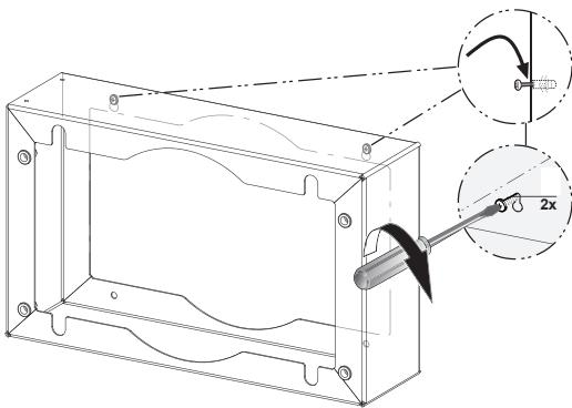
Hook the Rear Section as shown in the image above onto the upper screws and fully secure.
