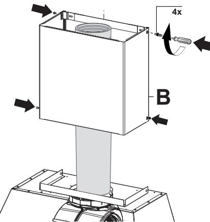
Secure the sides to the brackets by using the 4 screws .
