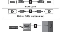
Connecting using an HDMI Cable (External Device (HDMI) / TV ARC/eARC)
